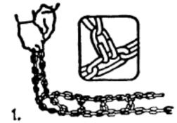
Lay chains out flat, remove all tangles. When chains are placed on the tyre, the cross hook eyes must face up (see the insert). Damage to your tyres could result if these hooks face against the tyre. Lay chain over the tyre, cross chain hooks up and the Lever fastener on the outside of the tyre. Tuck the spare length of chain under the tyre.
